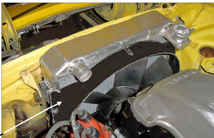
Aluminum radiator: shown with fan and shroud installed.
