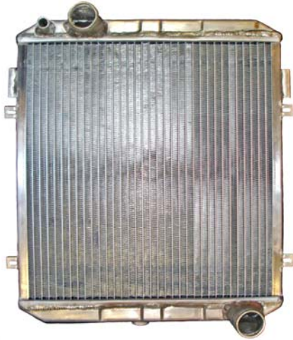
Aluminum radiator: shown with pressurized over flow and radiator hoses, however, without fan and shroud for clarity.
