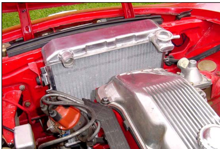
Aluminum radiator: shown without fan and shroud for clarity
