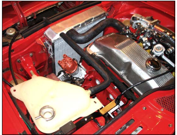
Aluminum radiator: shown with pressurized over flow and radiator hoses, however, without fan and shroud for clarity.
